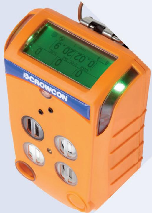
Gas-Pro is compatible with a wide range of sensor options including an Infrared (IR) sensor for detection of flammable gasses and CO<sub>2</sub> with guaranteed fast response, very low maintenance requirements, long lifespan and fail-safe operation. In addition Gas-Pro is also available with a PID sensor for detection of a wide range of VOCs perfect for the chemical industry especially if working with tanks containing solvents.
